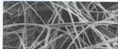
SEM of the P-BE filter media
